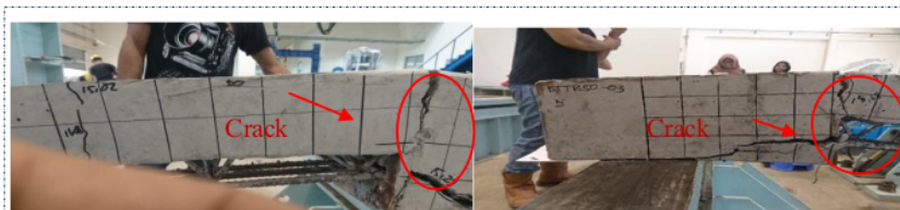
Figure 2. The crack at support.
